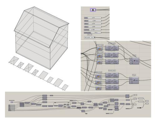
Fig. 6. 3D visualization of the sample building in Corso Umberto I according to the urban typologies parameters (top, left) and the complete algorithm and generative sequence (bottom) that figures out the 3D model, floor by floor and fit the building to each individual plot.
