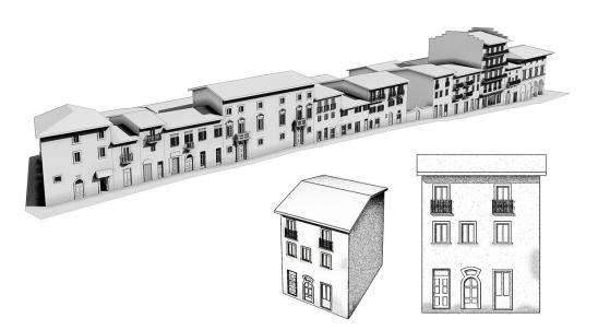
Fig. 8 .3D visualization of Corso Umberto I according to the façade composition and building composition (top) and extraction of the 3D model to be sampled and designed according to the façade type and the colour plan regulations (bottom).
