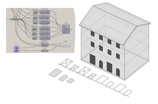
Fig. 7. 3D visualization of the sample building in Corso Umberto I according to the façade composition and opening parameters (right) and the algorithm and generative sequence (left) that figures out the 3D model, floor by floor, fitting the architectural composition for each façade. Model of Amatrice and a series of visualization and scenarios for each block according to state of the art before the earthquake.
