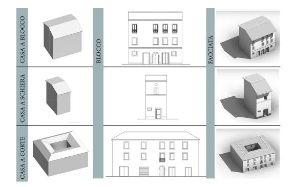
Fig. 4. The Pattern Book of Amatrice sets out an analytical study of the massing scale, proportions and details of individual buildings, to promote an organic reconstruction of the town, with appropriate architectural and urban tuning. The research presents an innovative protocol for territorial and urban simulation that produces the 3D model of the minimum intervention unit after the release of the reconstruction plan.
