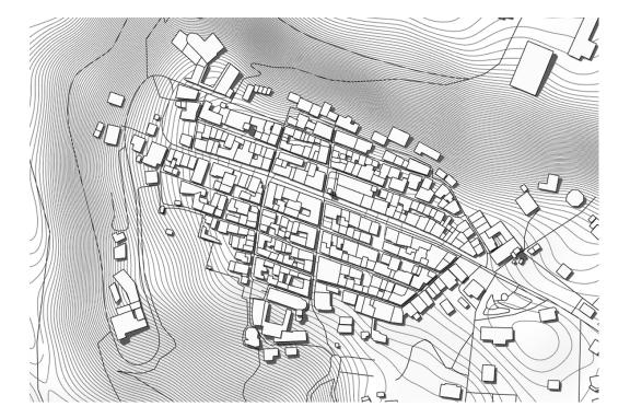
Fig. 1. Algorithmic modelling with Grasshopper and Elk to generate the Digital Ground Model of Amatrice and a series of visualization and scenarios from open source dataset. Maintenance of place character means simulate and visualize the typological, aggregative and functional solutions in respect of the regeneration of the social value of the places how it is expected by the community (fig. 2).
