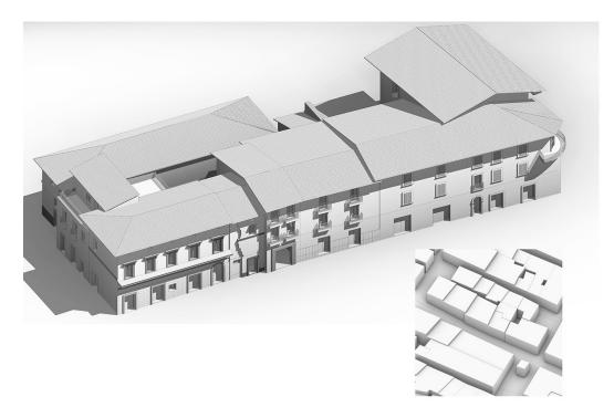
Fig. 2. 3D visualization of the HBIM model of the sample block in the centre of Amatrice generated according to the urban typologies and the architectural lexicon.
