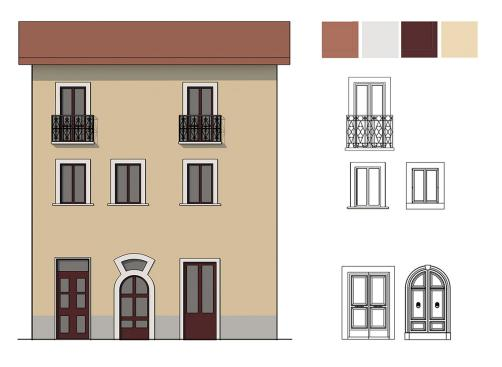
Fig. 10. 2D visualization of the façade composition, architectural lexicon, and colour palette according to the colour plan regulations.
