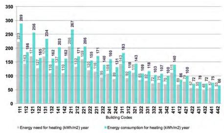
5.9 Energy need and energy consumption for heating (kWh/m<sup>2</sup> per year)
